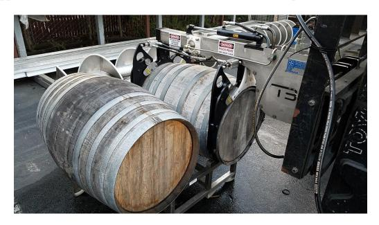
13. Once satisfactorily centered, lower the barrel to the drop point and slowly open the claws to release it. Raise claws clear of barrel and back up until claws are completely clear of barrels/racks. Repeat steps 9-13 as necessary.
