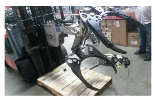
9. Once you are comfortable with the barrel picker operation, approach the barrel(s) to be moved.
