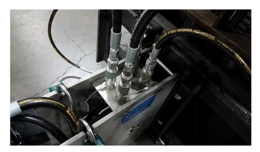
8. With the barrel picker attached and the hydraulic hoses connected, begin to manipulate the controls. Raise, tilt, open, close the picker as needed to gain a sense of control lever operation.
