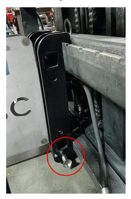
7. Connect the four hydraulic hoses from the forklift to the four quick-connect nipples on the barrel picker manifold. No need to connect hoses to any particular lever. Once connected, it is recommended that each control lever be labeled with its corresponding barrel picker function.
