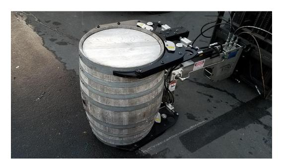
11. Raise the barrel and transport it to its destination. Rotate the barrel to desired orientation (vertical or horizontal). In this case, the destination is a horizontal barrel rack.
