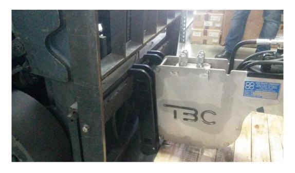
6. Insert locking pins (2 included) in the left and right sides of the frame attachment assembly. Pins should extend through the lower holes of the barrel picker frame hooks and through tabs on the fork frame.
