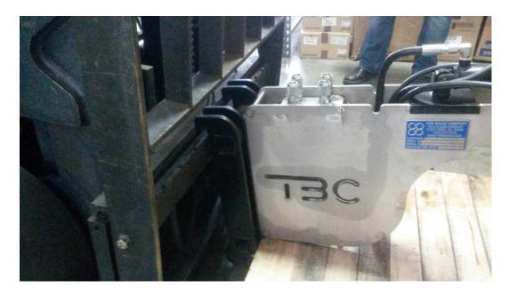
5. Slowly raise the fork frame until the barrel picker begins to raise. Check to make sure it is fully engaged on the fork frame.
