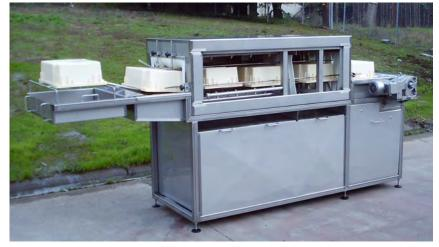
Zone Heated model has a second stage featuring a high temperature, high pressure rinse to ensure cleanliness. Each stage is internally screened and filtered to assure consistent results and minimize water consumption.
